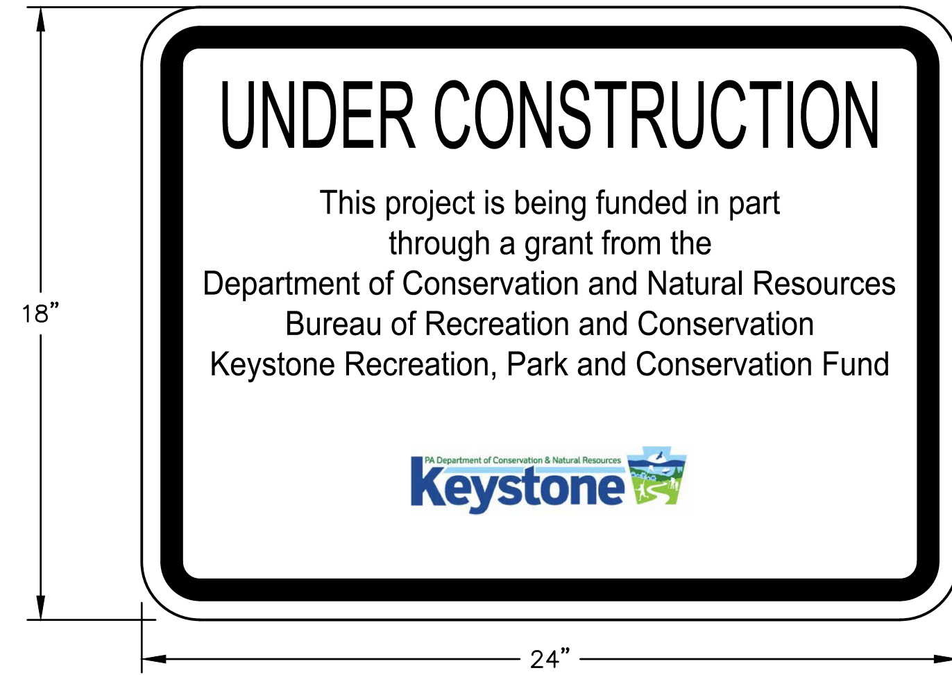
UNDER CONSTRUCTION DCNR FUNDING SIGN DETAIL ITEM 9000-0010 NOT TO SCALE
